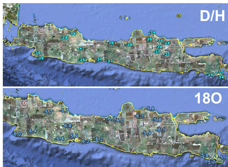
Figure17: Calculated D/H and ^{18}\text{O}/^{16}\text{O} isotope ratios of groundwater in the Java region
